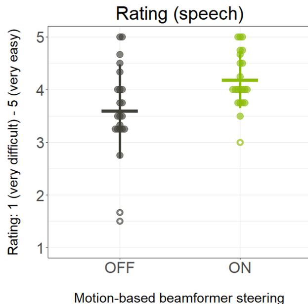
Figure 2. Subjective rating results for tasks related to speech. Ratings were done on a 5 point Mean Opinion Score (1 = very difficult, 5 = very easy). Horizontal lines indicate means and whiskers stretch to the 10<sup>th</sup> percentile.
